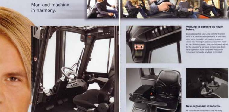
New ergonomic standards. All controls and instruments are perfectly located for the convenience of the operator. Toggle switches for accessories such as lights. work lamps or wipers are integrated into the overhead guard leaving an unobstructed view to the fork tips. Important truck status
